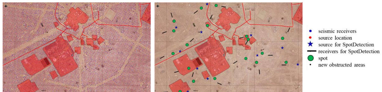
Figure 1 Left: Field A with seismic 3D layout and new obstructed areas. Right: Field A with the SpotDetection layout, the spots locations, and the new obstructed areas.
