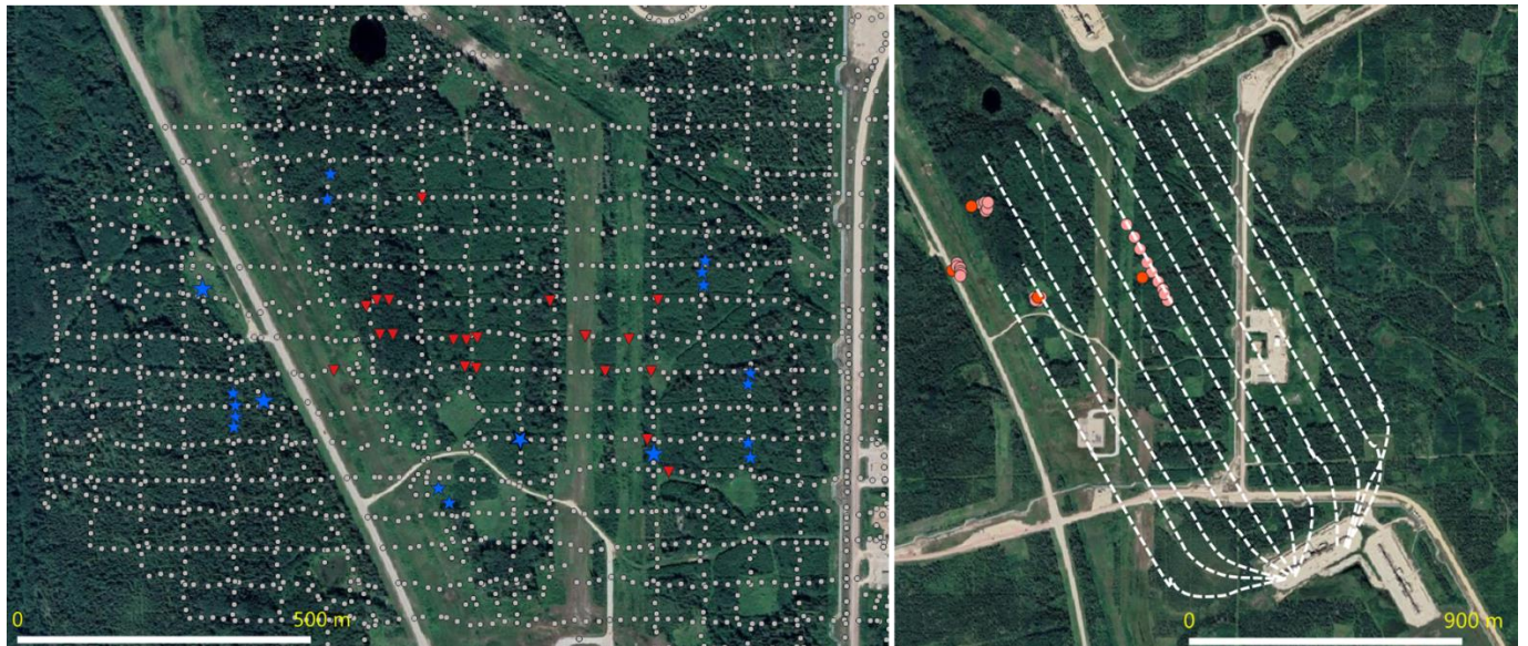
Figure 1 – Left: Seismic acquisition design with both 3D permanent design in grey (1700 shots casing and 2500 buried geophones taking several weeks to operate) and the light focused acquisition system (19 sources locations – blue stars and 20 geophones recordings – red triangles operated in a 5 days). Right: Monitoring map associated with the light and focused acquisition design. The dashed white lines stand for the horizontal well design. The four red dots are the original four spots to be monitored on the area. The 20 pink dots are the common-mid point locations that were acquired in addition during the June acquisition campaign to validate the operational model.
