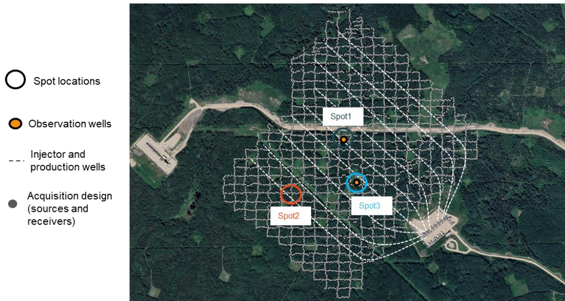
Figure 1 Blind-test scenario on PAD101 North. Spot locations have been defined over observation wells in order to correlate the detections of the steam chamber variations. Reservoir depth is 450m.
