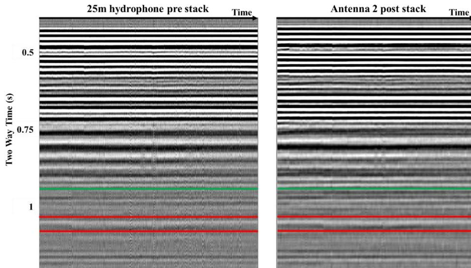
**Figure 3** 132 days of continuous data with 50 sweeps per day: single 25m hydrophone (left); daily 3-hydrophone antenna stack (right). Gas storage is indicated in green and oil reservoir top and base in red.
