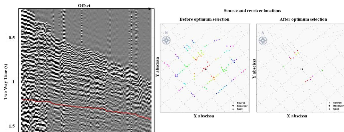
**Figure 1** A common spot gather example with oil reservoir in red (left). Source-receiver pairs before (middle) and after optimum selection (right).
