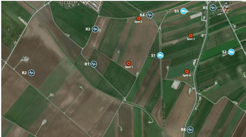
**Figure 2** Survey design including receiver antennae (R1 to R6, in dark blue), sources (S1 to S3, in light blue) and spots (Spot 1 to 4, in orange).
